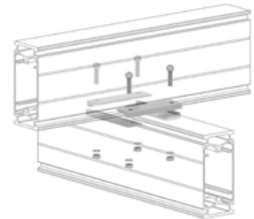
SPX410 Cross joint in 20 micron anodized aluminium for overlapping aluminium beams
